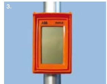
1. Pilot installation on ENION S.A. distribution station, Krakow, Poland | 2. Status – voltage on | 3. Status – voltage off.
